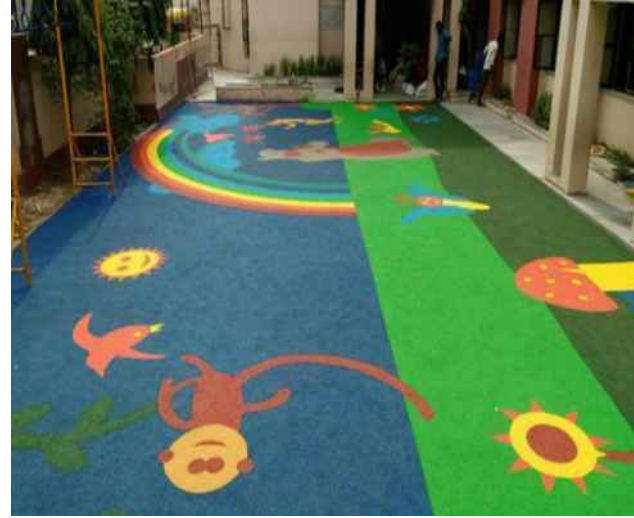
SBR (Styrene Butadiene Rubber) Thickness Available : 36mm, 25mm, 20mm & 15mm
